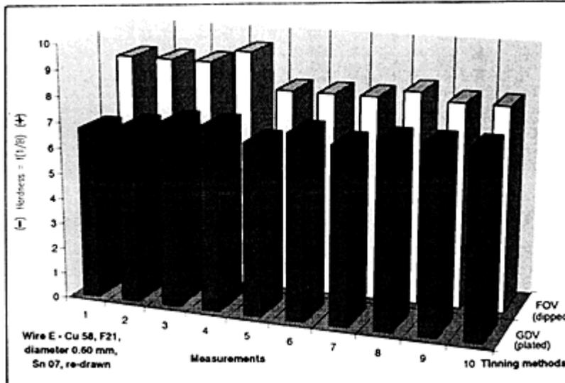
There are 2 wire samples laying under a swinging roll-pendulum. After about 440 pendulum movements the roll stops. The depth and the width of the pressed area on the wire can give a comparative indication for the hardness of the surface layer. All measurements only give an indication.
