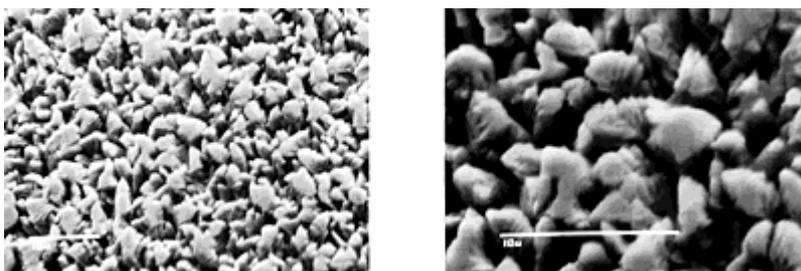
Electroplated tin- or tin/lead-alloys grow in a column crystalline structure (rod-shaped, stalk-shaped). There are cavities between the single crystals. The surface itself is porous.
