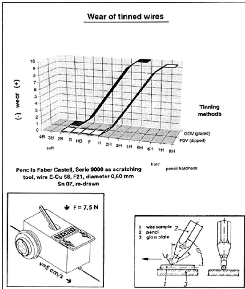
Therefore pencils with different degrees of hardness are fastened in a specific device, which runs over the wire-surface. Increasing the degree of pencil-hardness results from a certain point to a peeling of the tin coating (Scratch hardness testing).
