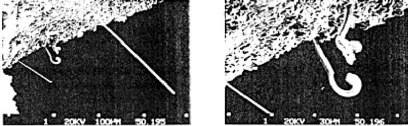
Whiskers are fine, capillary single crystals consisting of different materials, which may grow out of the metallic layer.
