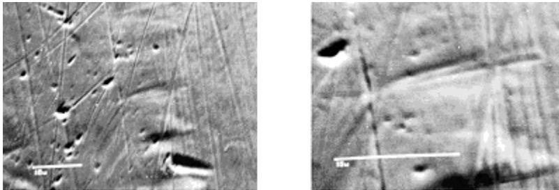
The tin coating is applied directly from the molten bath and has a dense and smooth surface with a homogeneous structure.
