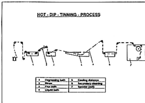
Fig. 2 The Hot-Dip Tinning Process
