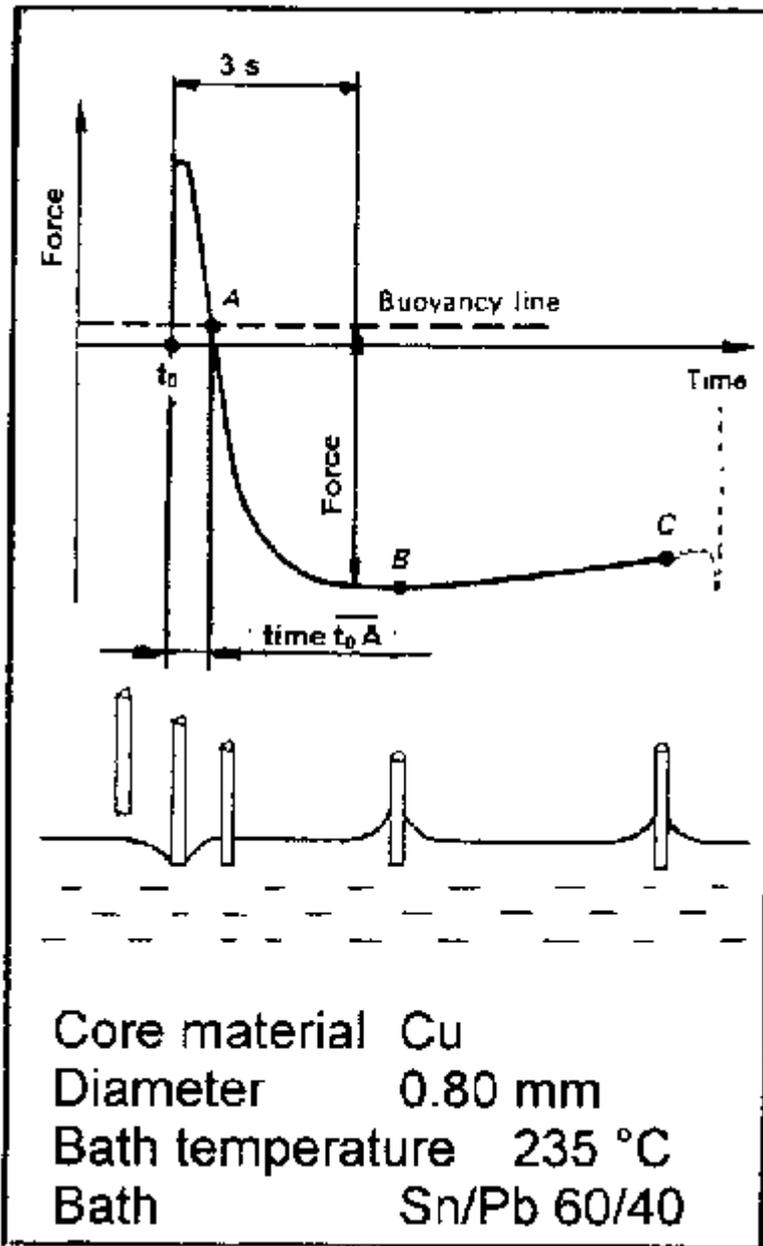
Fig. 7 Solderability Test by the Wetting Balance Method
