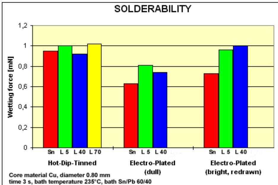
Fig. 9 Wetting Force of Coated Wires
