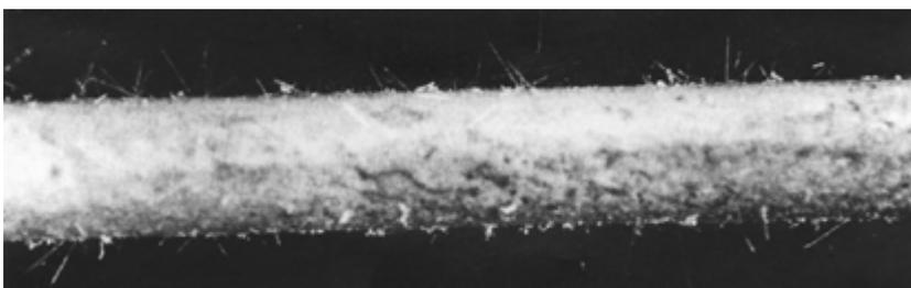
Fig. 11 Whiskers on a Coated Wire [9]
