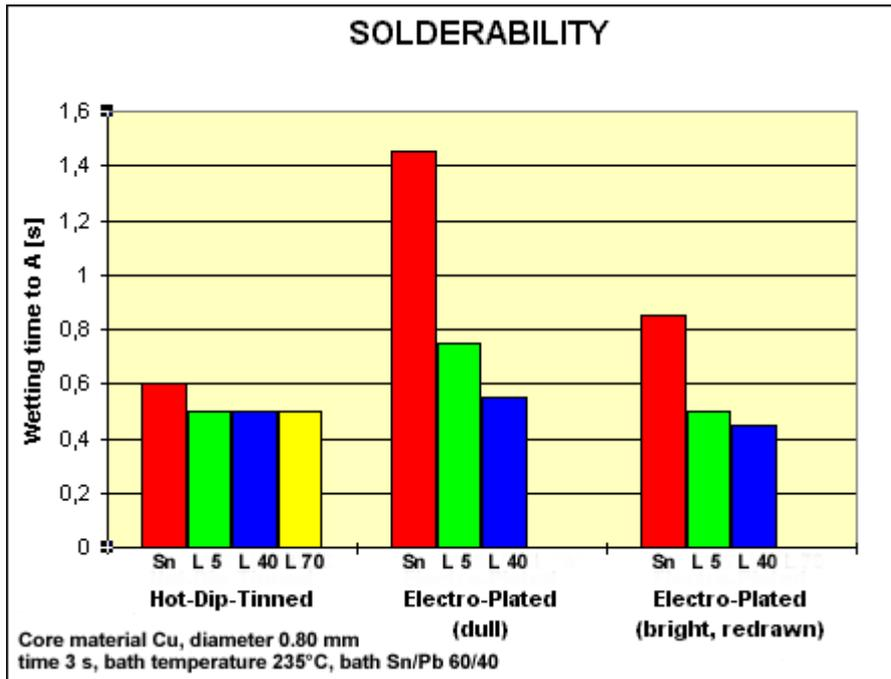
Fig. 8 The Wetting Time of Coated Wires
