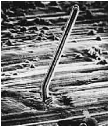
Fig. 10 Scanning Electron Micrograph (SEM) concerning a whisker growth out of an electroplated tin layer [9]
