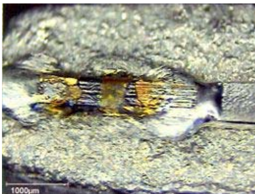
Fig. 11: Soldering not ok
